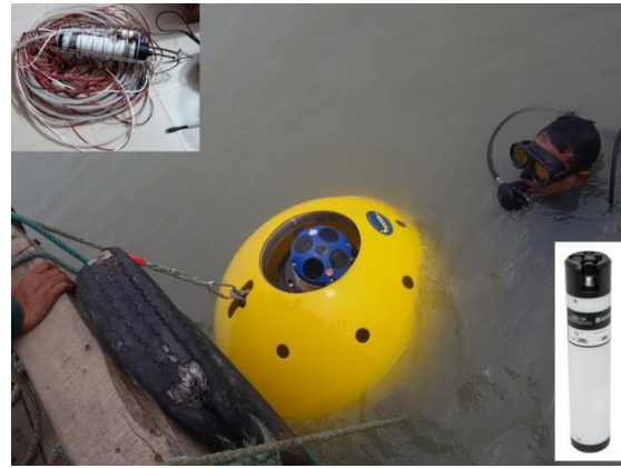
Deployment of the ADCP (inset Turbidity sensor)
