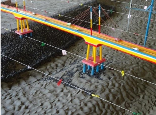
Local scour in the vicinity of bridge pier and revetment
