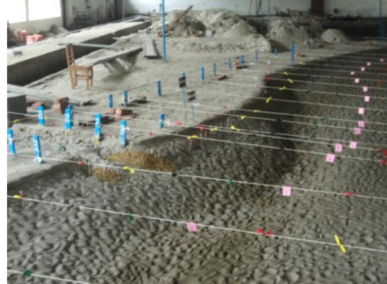
Local scour in the vicinity of bridge pier and revetment
