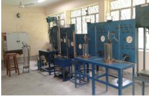
Triaxial Shear Test Apparatus used for determining Shearing strength of soil
